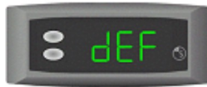
Figure 15. Display during defrost, drain down, or recovery
